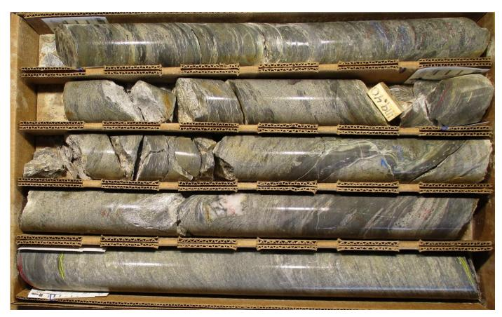
Figure 3: Massive sulphide mineralised interception at hole BMZ79 from 417.3 metres to 420.28 metres downhole depth. Sulphide mineralisation both follows cross-cut primary foliation in the hosting rhyolite rock. Sphalerite is pale brown; chalcopyrite bright yellow. Pyrite completes the visible sulphide assemblage
