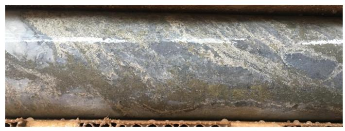
Figure 4: Closer view of Massive sulphide mineralised interception at hole BMZ79 at 456 metres downhole depth. Sulphide mineralisation both follows cross-cut primary foliation in the hosting rhyolite rock. Sphalerite is pale brown; chalcopyrite bright yellow. Pyrite completes the visible sulphide assemblage
